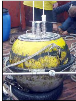
Figure 14 The buoy after five weeks at sea. The fouling is limited to a biofilm.
