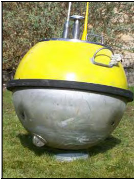
Figure 13 The buoy equipped with the ACM before deployment. The transducers can be seen as dark circles at the left and right of the bottom half of the buoy.
