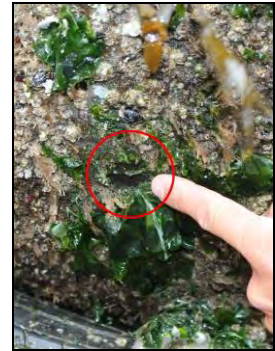
Figure 16 A view of the front facing transducer after fourteen weeks. The transducer is visible as a black area within the red circle.
