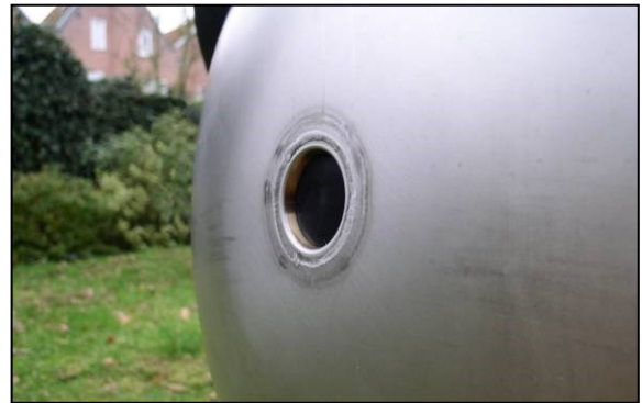
Recessed transducer in the hull.
