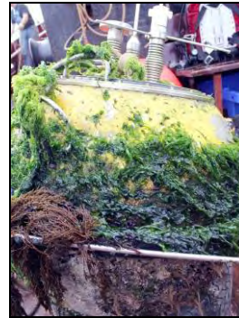
Figure 15 The buoy after fourteen weeks at sea. Green fouling is mainly present on the top half; brown fouling and small shells are present on the bottom half.
