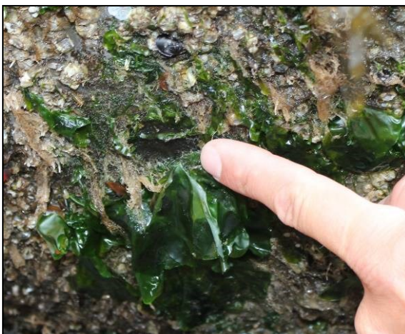
Transducer hardly visible, still measuring.
