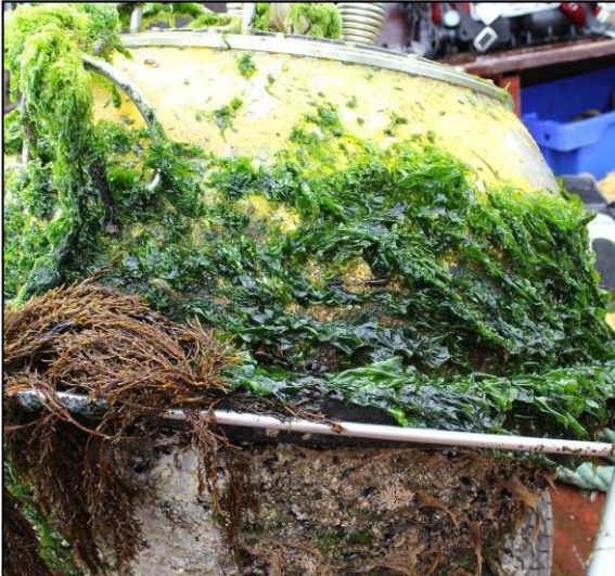
Fouling after fourteen weeks at sea.
